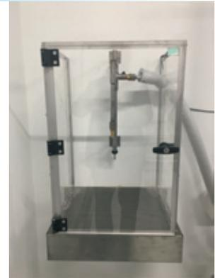
Pressure tank with CryoSafe, "deadman's" button, manually withdrawing liquid nitrogen and stainless steel filling cabinet with plexiglass doors and drip tray
