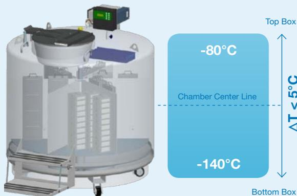
Temperature gradient within storage space (top box to bottom box) is between 2°C and 5°C
